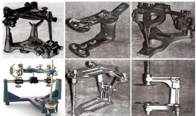
Figs. 9A to F: (A) Terrell's precision coordinator, (B) Hanau crown and bridge articulator, (C) Phillips oclusoscope, (D) McCollum gnathoscope, (E) Stephan articulator and (F) Fournet articulator Fonte: Jain,2016
