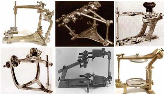
Figs. 6A to F: (A) Gysi adaptable articulator, (B) Gysi simplex articulator, (C) Luce articulator, (D) Eltner articulator, (E) Halls alligator and (F) Hall's anatomic articulator Fonte: Jain,2016
